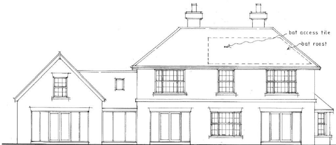
south west elevation
